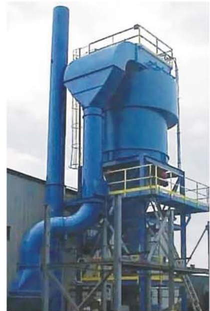
Tangential inlet design for low bulk density dust
